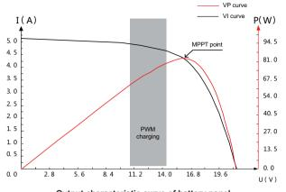
Output characteristic curve of battery panel
